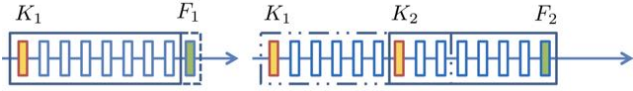
Figure 2. Left: when sufficient feature points are tracked to a new frame c , the local window attached to the keyframe K_1 expands to include F_1 . Right: when insufficient features are tracked, a new keyframe K_2 will be selected, and a new local window expands to cover F_2 .
